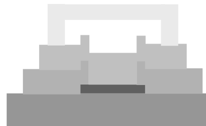
(d) Bonding of a PDMS upper plate with a chamber (A-A section)
